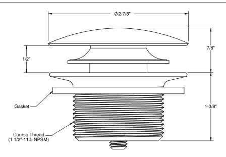
Figure 1. Drain in **OPEN** position
